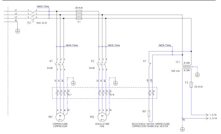
G5C 250 (460/3/60) POWER WIRING DIAGRAM - Cod. 714.003.02.00 - Rev. 03 - 02.05.02
